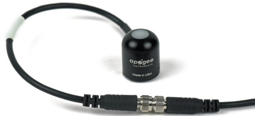
In-line cable connectors are installed 30 cm from the head (pyranometer pictured)
