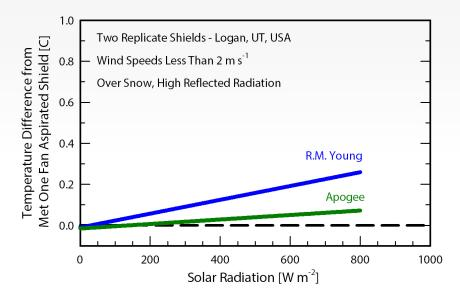
The performance of model JTS-110 and model 43502 fan-aspirated shields relative to a model 076B fan-aspirated shield.
