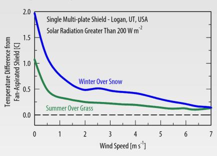
Naturally-aspirated shields are subject to significant measurement errors when wind speeds are less than 3 m s<sup>-1</sup>. Errors increase when snow covers ground surface.
