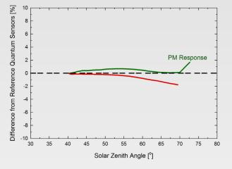
Mean cosine response of seven Apogee JSQ-500 quantum sensors. Cosine response measurements were made on the rooftop of the Apogee building in Logan, UT. Cosine response was calculated as the relative difference of JSQ-500 quantum sensors from the mean of replicate reference quantum sensors (LI-COR models LI-190 and LI-190R, Kipp & Zonen model PQS 1). The red data are AM measurements; the green data are PM measurements.
