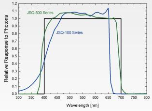
Mean spectral response measurements of six replicate Apogee JSQ-100 and JSQ-500 series quantum sensors. Spectral response measurements were made at 10 nm increments across a wavelength range of 300 to 800 nm in a monochromator with an attached electric light source. Measured spectral data from each quantum sensor were normalized by the measured spectral response of the monochromator/electric light combination, which was measured with a spectroradiometer.
