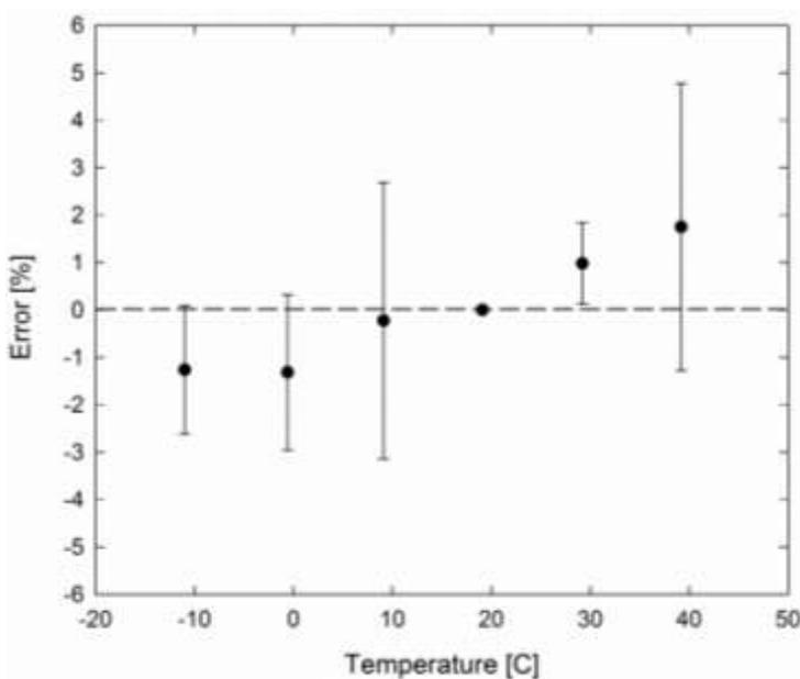
Mean temperature response of eight replicate sensors (**errors bars represent two standard deviations above and below mean**).
