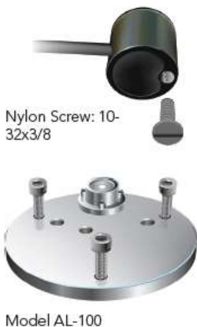
To minimize azimuth error, the sensor should be mounted with the cable pointing toward true north in the northern hemisphere or true south in the southern hemisphere. Azimuth error is typically less than 1 %, but it is easy to minimize by proper cable orientation.
