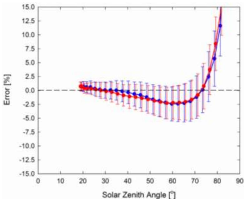
Mean cosine response of twenty-three replicate sensors (**error bars represent two standard deviations above and below mean**). Cosine response measurements were made by direct side-by-side comparison to the mean of four reference thermopile pyranometers, with solar zenith angle-dependent factors applied to convert total shortwave radiation to PPF. Blue points represent the AM response and red points represent the PM response.
