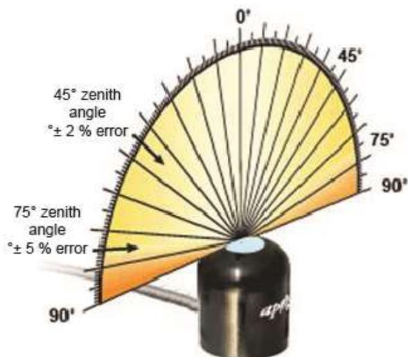
Directional, or cosine, response is defined as the measurement error at a specific angle of radiation incidence. Error for Apogee SQ series quantum sensors is approximately  $\pm 2\%$  and  $\pm 5\%$  at solar zenith angles of  $45^\circ$  and  $75^\circ$ , respectively.
