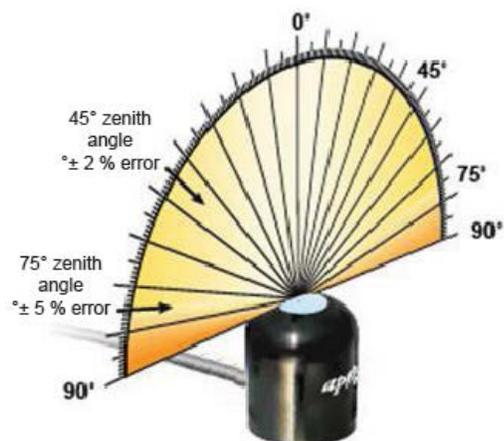
Directional, or cosine, response is defined as the measurement error at a specific angle of radiation incidence. Error for JSQ series quantum sensors is approximately  $\pm 2\%$  and  $\pm 5\%$  at solar zenith angles of  $45^\circ$  and  $75^\circ$ , respectively.
