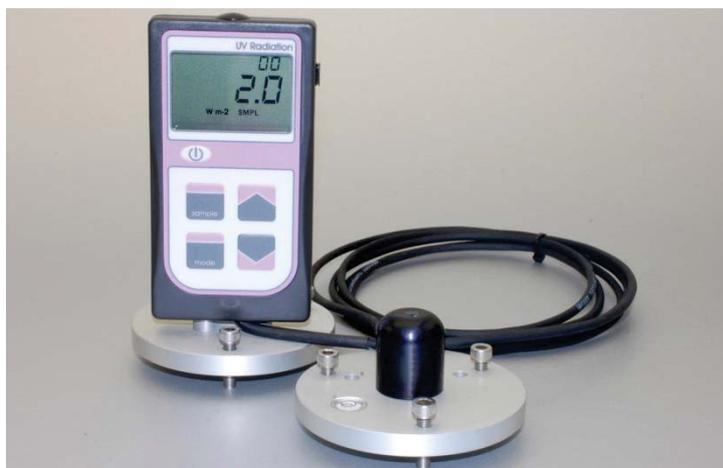
The ultraviolet meter measures and displays instantaneous readings of the ultraviolet radiation between 250 and 400 nanometers (nm) in  $\mu\text{mol m}^{-2} \text{s}^{-1}$  (micromoles of photons per square meter per second) or Watts. The self-cleaning dome-shaped head of the **JMU-200** prevents water accumulation. The sensor head is potted solid to prevent internal condensation in humid environments.
