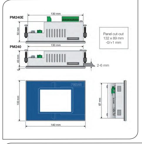
The PM240 is a 320x240 pixel touchscreen terminal with a 3.5" colour TFT display. It allows the user to display data from up to eight PyroBus sensors and configure each sensor individually. The configuration parameters include emissivity setting, signal averaging, peak or valley hold processing and reflected energy compensation.
