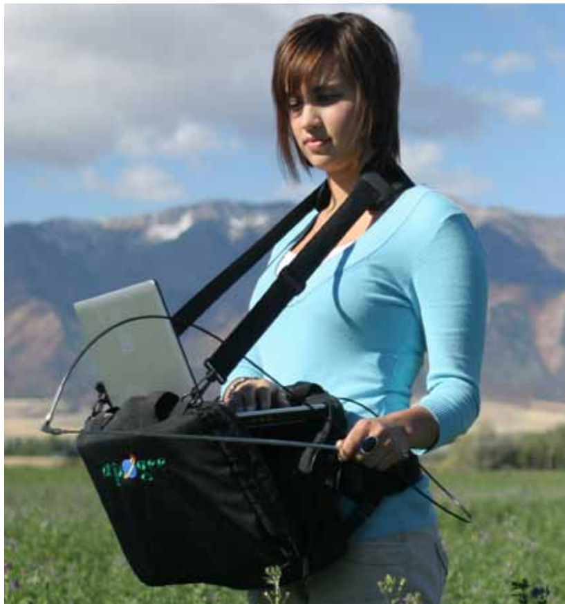
Model JPS-100 with carrying case and reflectance wand
